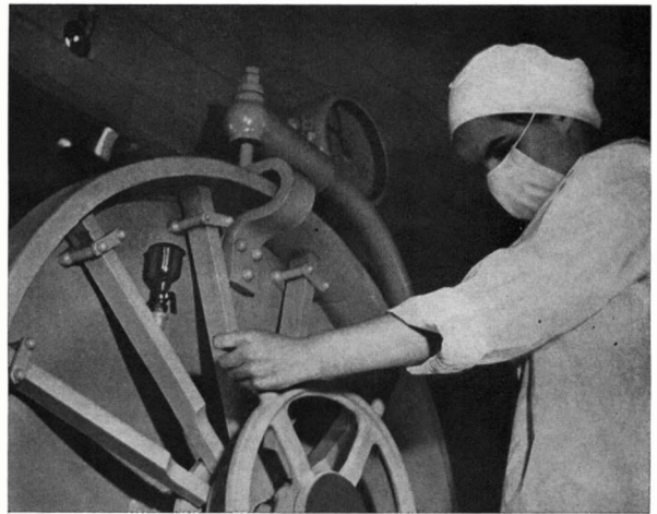
A lab assistant makes sure the autoclave is tightly sealed before flooding bottles inside with live steam. Like the other assistants, she always wears a mask on the job.
