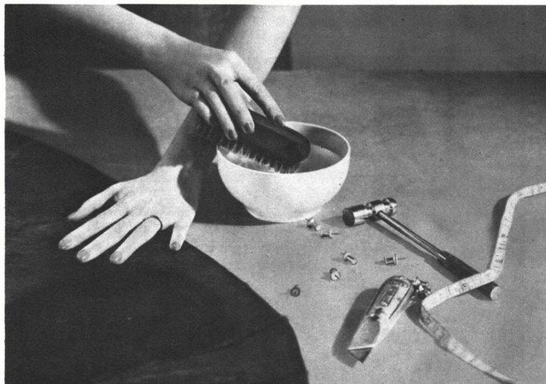
Blocking: Using brush and cool water she dampens the leather side. She outlines the pattern of the cape upwards and sideways, she tacks and pulls the dampened fur—stretching it so that it extends slightly beyond the edge of the pattern on all sides.
